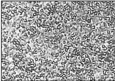
Finegrain-hardmetal structure Ultra-micro-grain, grain size 0–0.5 micron
