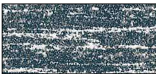
Original HSS-milling cutter • brittle construction • limited strength
