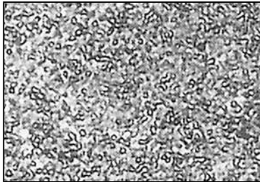
Finegrain-hardmetal structure Ultra-micro-grain, grain size 0–0.5 micron
